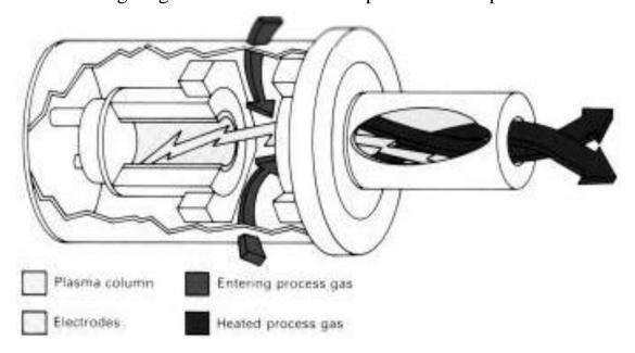
The temperature a few feet from the torch can be as high as 5,000-8000° F. Because of these high temperatures the waste is completely destroyed and broken down into its basic elemental components. There are no tars or furans. At these high temperatures all metals become molten and flow out the bottom of the reactor. Inorganics such as silica, soil, concrete, glass, gravel, etc. are vitrified into glass and flow out the bottom of the reactor. There is no ash remaining to go back to a landfill.
